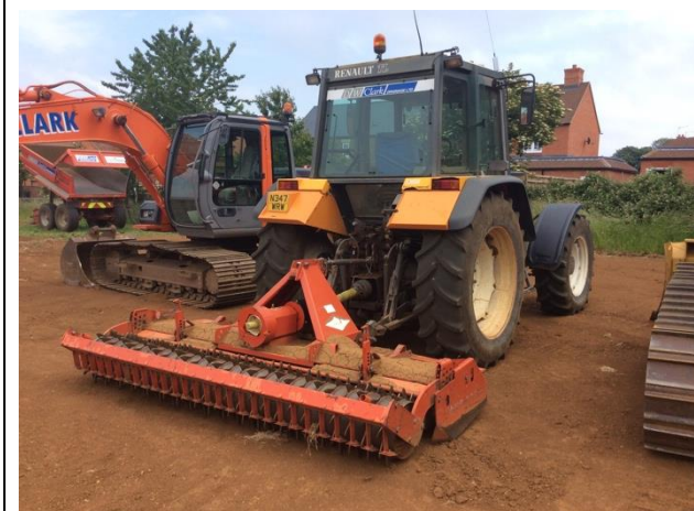
Figure 11: The drainage contractor has a number of key pieces of equipment on site to carry out final cultivation operations to break up the larger soil aggregates to promote a more friable profile and finer surface soil tilth.
